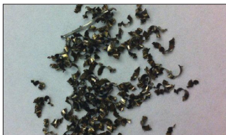
Regular curled chips. Shape and length depend on end mill geometry and cutting data.
